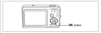
You can use the camera as a clock. With the camera turned off, press and hold down the **OK** button to display the clock on the LCD monitor.
