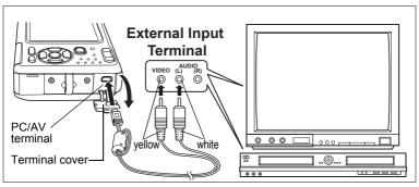
By using the AV cable, you can capture and play back images on equipment with a video IN jack, such as a TV. Make sure the camera and TV are turned off before connecting the camera to the TV.
