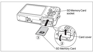
This camera uses an SD Memory Card. Captured images and sound files are saved on the SD Memory Card if a card is inserted in the camera. They are saved in the built-in memory if a card is not inserted. (p.32)
