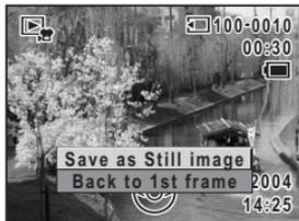
The image displayed on the LCD monitor is saved as a 320 × 240-pixel still picture.
