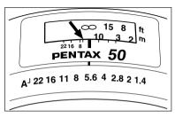
When taking infrared pictures with infrared film and either a "R2" or "02" filter, it is necessary to adiust the focus because the point of focus is not the same with infrared light as it is with visible light. As shown above, memorize the focusing point on the lens distance scale when viewed through the viewfinder and turn the focusing ring until the point you memorized aligns with the infrared index.
