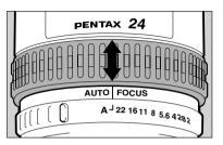
FA\* 24mm f/2 lens has a focusing ring which provides autofocus and manual focus settings. Push the focusing ring or pull it towards you to set the autofocus or manual focus mode respectively.
