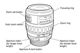
\* An FA Zoom lens without the power supply contacts on its mount does not have the zoom set button and auto zoom switch.
