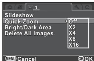
**3** Use the four-way controller (▲▼) to select [Bright/Dark Area], and use the four-way controller (◀▶) to select  or .
