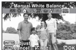
**2** Under the light you wish to measure the white balance of, fully display a white sheet of paper on the monitor, or select a white area as the subject.
